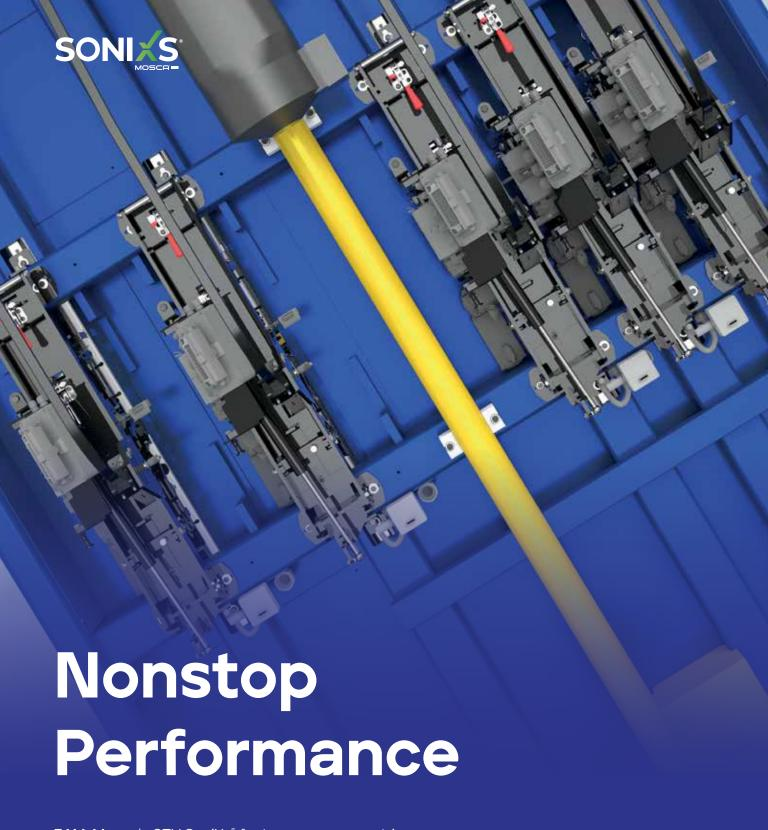
EAM-Mosca's CTV SoniXs® features an asymmetric platen with five strap heads to accommodate the widest variety of load sizes and strap patterns. Strap placements range from 9" - 56.5".
