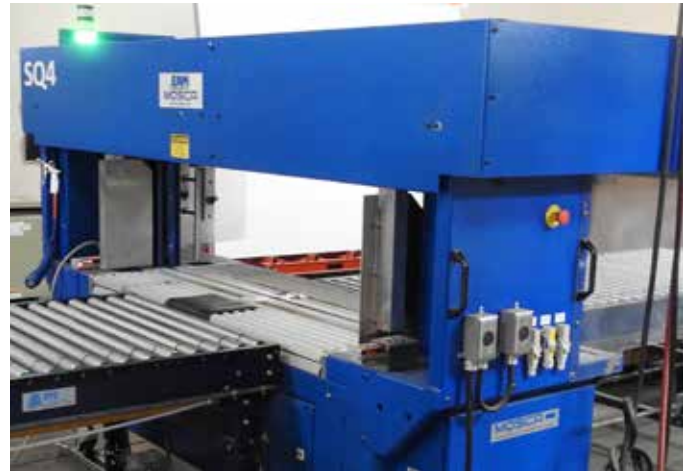
An SQ4 SoniX automatic squaring bundler by EAM Mosca combines high-speed and flexibility to strap a wide variety of bundle sizes.
